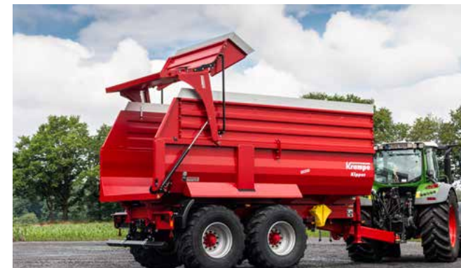
For our SK models, a lot of extensions in the height of 40, 60 and 80 cm are available whereby the 80 cm extensions can additionally be supplemented with a 20 cm high aluminium extensions.
