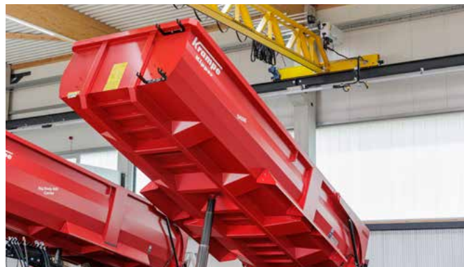
The SK body is characterised by heavy beams under the body and a heavy underfloor cylinder.
