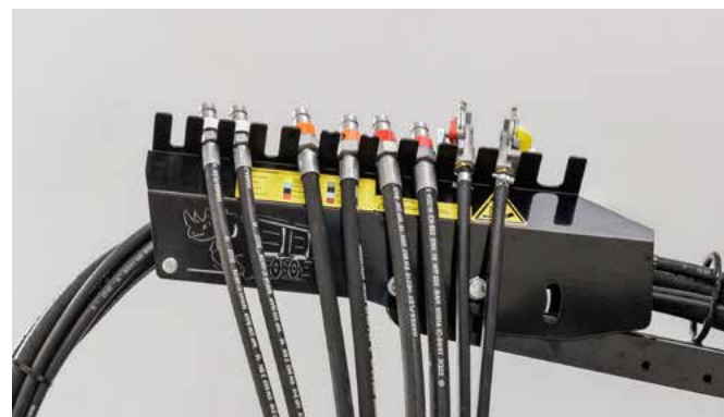
The hose holder ensures order and is adjustable in length and height by a few handles.
