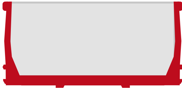
Conical body with flat floor sheet. Through optional volume extensions, the volume for light goods can be increased.
