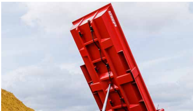
The HD body is characterised by heavy beams under the body and an underfloor cylinder.
