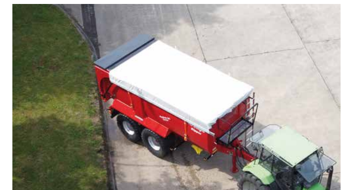
The roll-over tarp can directly be fastened on the body. The use of the roll-over tarp is also problem-free possible with the silage extensions, available for the SK models.
