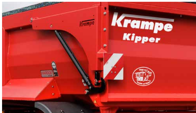
Hydraulically opening rear tailgate with automatic lateral pressing system with locking block valve, safety ball valve and closing hook stop mode which can override the closing hooks if necessary.
