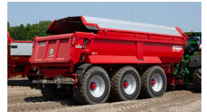
The high-quality aluminium folding cover can be opened or closed in only approx. 20 seconds and is available up to a length of 9.0 m.
