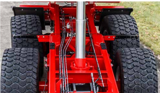
With 600 tyres, an outside width of 2.55 m is possible due to the cranked running gear with a tracked width of 1.95 m.
