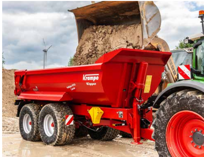
The front protection hood protects the front press and towing device against damages through falling load.
