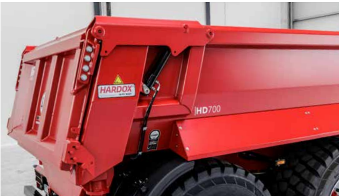
The robust hydraulic rear tailgate with protected hydraulic cylinders is additionally pendulum mounted.
