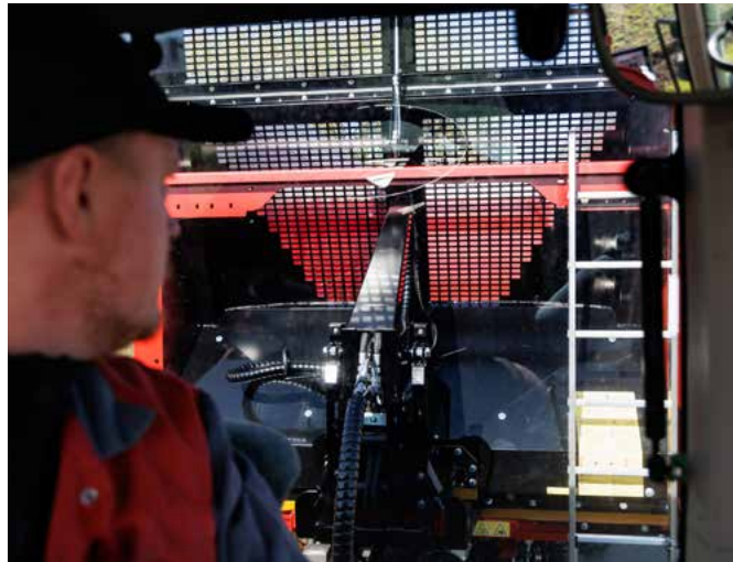
The driver always has a good view on the load due to the extensive lattice look of the push blade.
