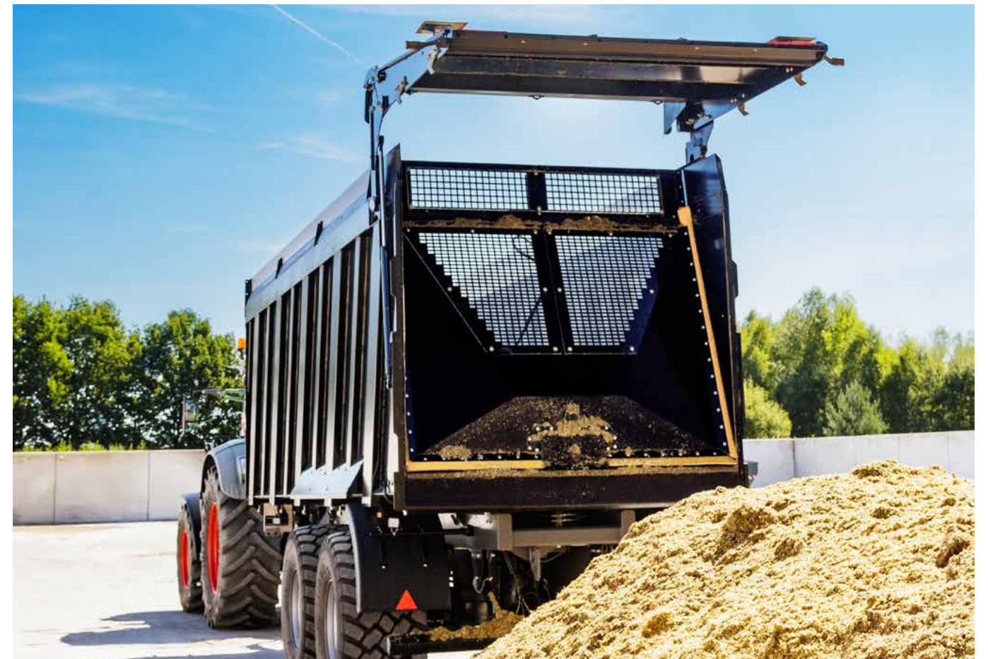
Our RamBody 750 unloads 40 m 3 silage maize in only approx. 45 seconds at 100 l/ minute.
