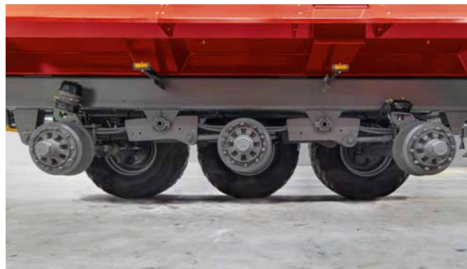
For the RamBody 900, we use 36 t parabolic springs with trailing arms and dynamic compensation with a wheelbase of 1.55 m.
