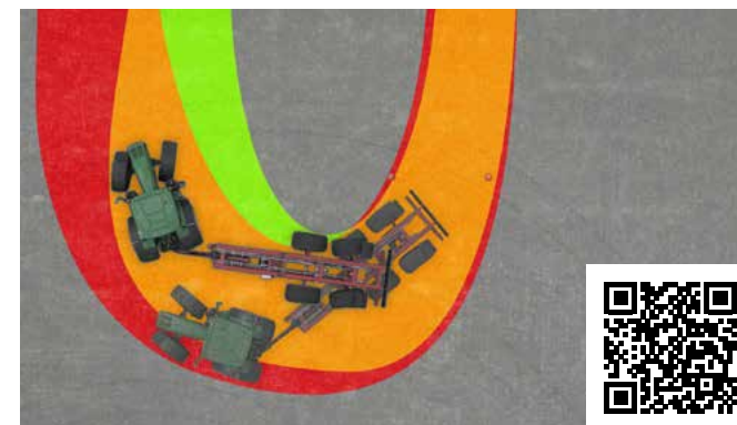
Our electronic sensorless forced steering enables the trailer to steer actively. This ensures a significantly improved vehicle manoeuvrability.
