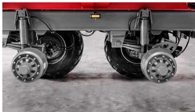
Also Krampe supplies hydraulic running gears. The standard protection tubes protect the double chromed piston rods against stone impacts.
