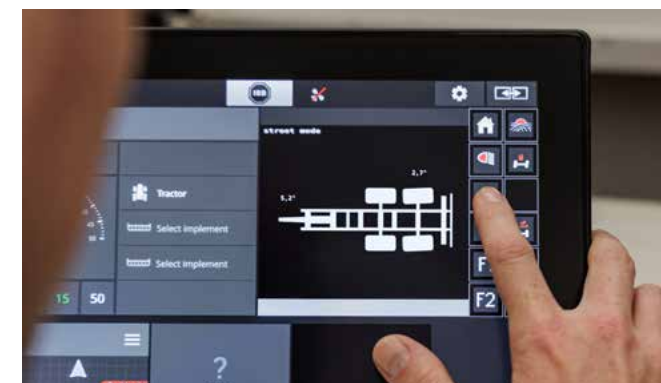
By means of an ISOBUS control, we have implemented the operation via the terminal of the tractor for forced steering.
