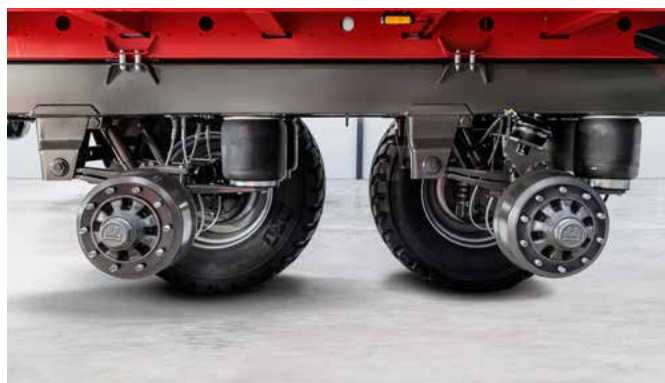
Pneumatic running gears are becoming more and more popular and are partly already offered as standard. The two-bladed pull rods and the large air bellows ensure an excellent engine smoothness and a stable driving behaviour.
