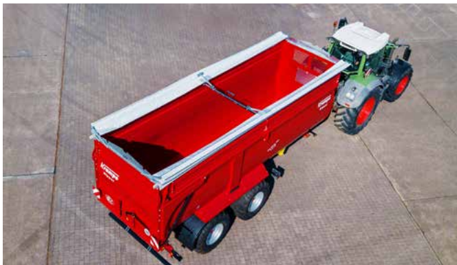
The Fliptop covering system opens and closes hydraulically to both vehicle sides.
