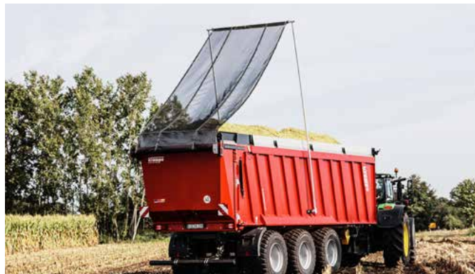
The laterally pivoting alu brackets open and close the net covering.
