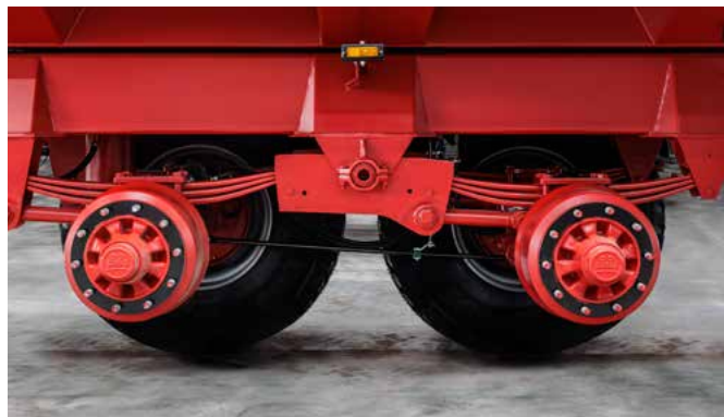
The 32 ton parabolic springs fitted as standard on the RamBody 750 guarantee a high ground clearance. Available with a wheelbase of 1.55 and 1.81 m.
