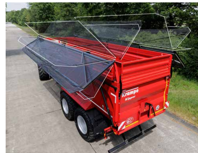
The two-sided hydraulic Krampe TwinTop cover opens and closes within only approx. 15 seconds and can easily be actuated from the driver's cab.
