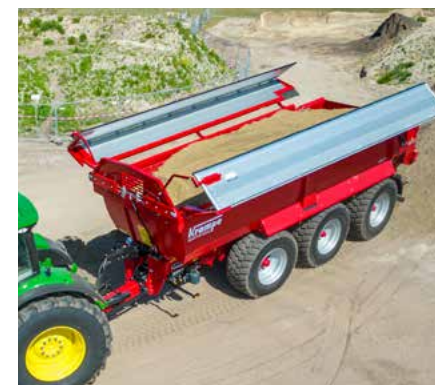
The high-quality aluminium folding cover can be opened or closed in only approx. 20 seconds and is available up to a length of 9.0 m.
