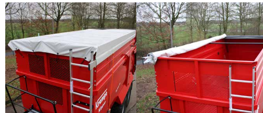
Roll-over tarps are an easy but proven system for load securing. The tarpaulin can quickly and easily be rolled and secured by means of the winding board.
