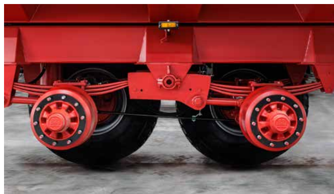
For the larger BigBody models, we use 24 – 36 t parabolic springs with trailing arms and dynamic compensation with a wheelbase of 1.36 - 1.81 m. The wide spring centre increases the stability off-road, especially on the vehicles with high centre of gravity.
