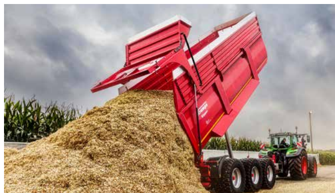
The 80 cm high steel extensions can be extended by further aluminium extensions with a height of 20 cm.
