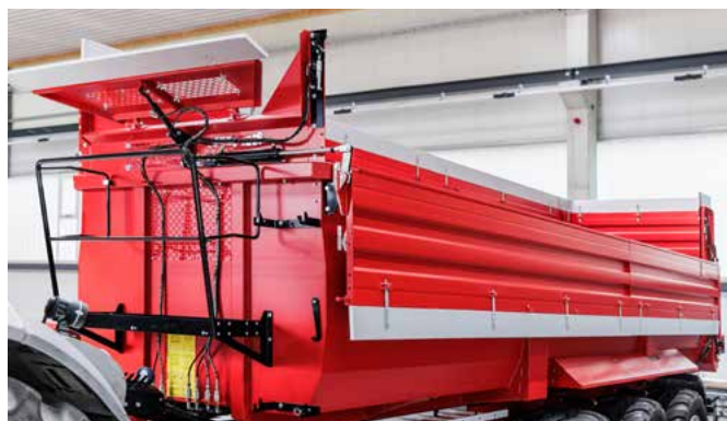
The laterally foldable extension sidewalls can be actuated hydraulically.
