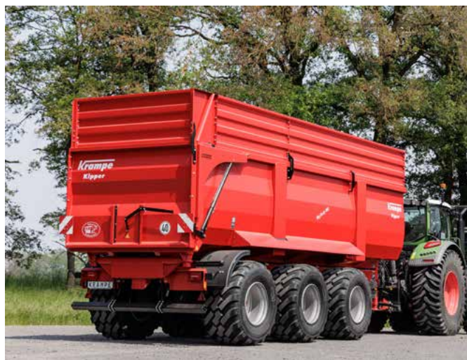
Silage extensions are available as steel silage extensions with a construction height of 60 or 80 cm.
