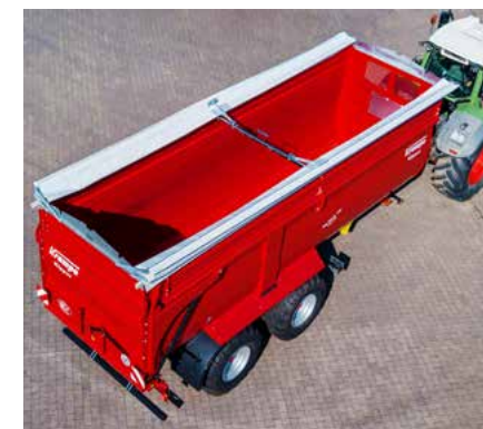
The Fliptop covering system opens and closes hydraulically to both vehicle sides.
