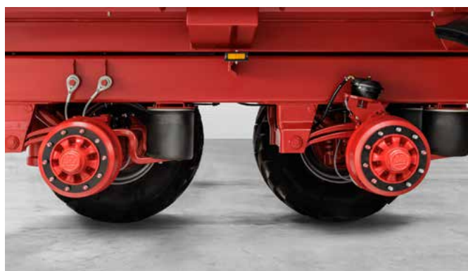
Pneumatic running gears are becoming more and more popular and are partly already offered as standard. The cranked two-bladed pull rods with the large air bellows ensure an excellent engine smoothness and a stable driving behaviour. By venting the air bellows, the vehicle automatically lowers during tipping and increases thus the stability
