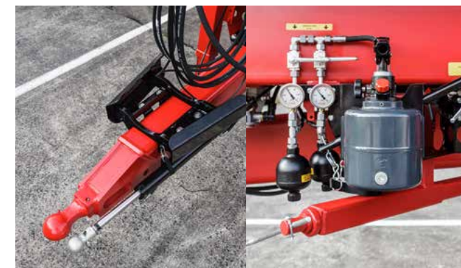
BPW forced steering: The double-acting master cylinder is situated at the front at the towing device, on the left and right in travelling direction for the Tridem, hydraulic system completely with hand pump, manometers and nitrogen accumulators, coupling points on the tractor according to standard proposition (ISO 26 402).
