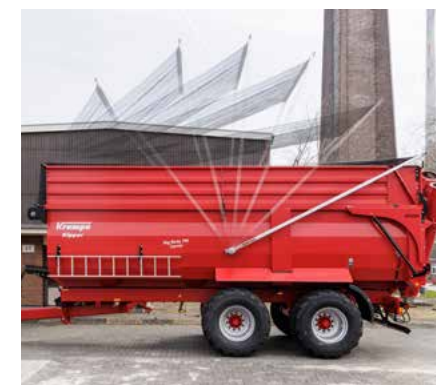
The laterally swivelling aluminium brackets open and close the net covering. The external vehicle width can exceed 2.55 m, it is permissible according to German Traffic Road Regulations.
