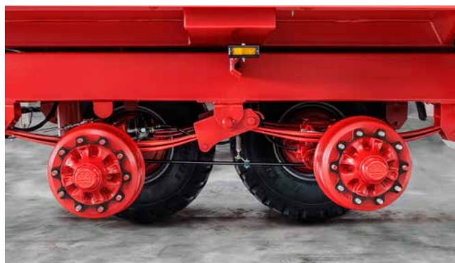
The 20 ton parabolic springs fitted as standard on the BigBody 500 and 540 guarantee a high ground clearance.
